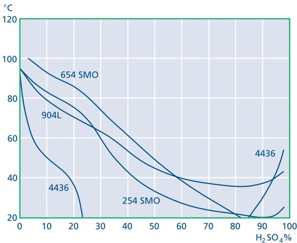
Fig. 1. Isocorrosion curves, 0.1 mm/y, in pure sulphuric acid.
