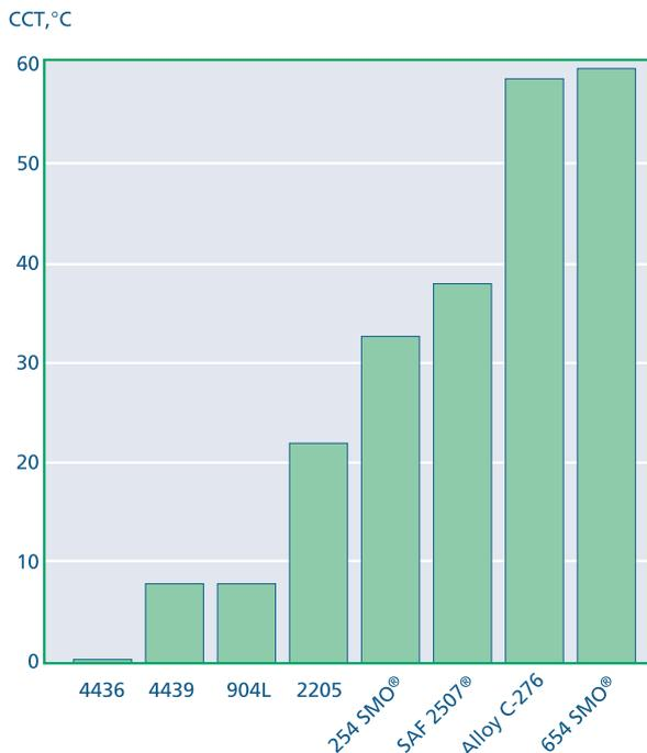
Fig. 7. Critical crevice corrosion temperatures (°C) for some stainless steels in 6% FeCl<sub>3</sub>. Testing according to MTI-2.
