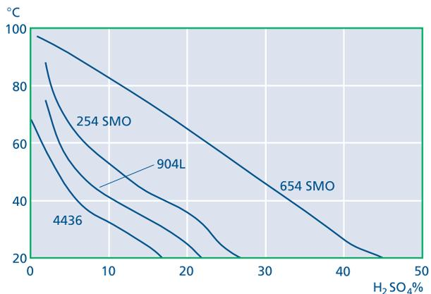
Fig. 2. Isocorrosion curves, 0.1 mm/y, in sulphuric acid containing 2000 ppm chloride.
