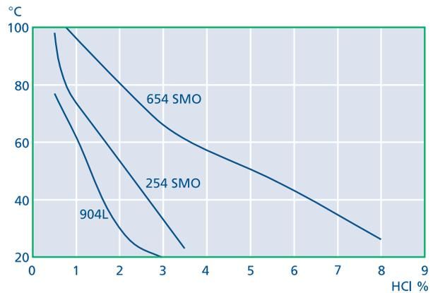
Fig. 3. Isocorrosion curves, 0.1 mm/y, in pure hydrochloric acid.
