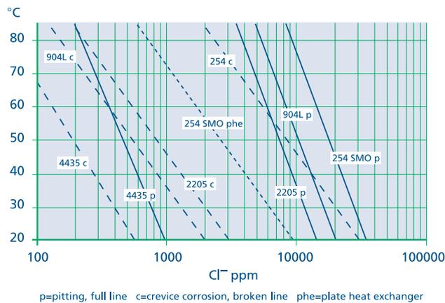
**Fig. 9.** Risk of pitting and crevice corrosion on high alloyed stainless steel in water of different chloride content or temperature.
