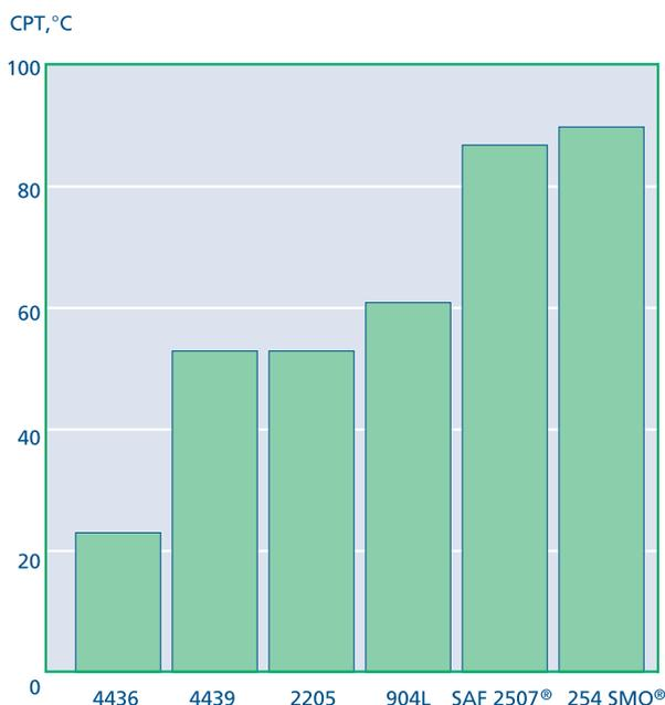
**Fig. 6.** Critical pitting corrosion temperature (CPT) for different stainless steels. Measured in 1 M NaCl according to ASTM G150, using the Avesta Cell.
