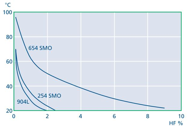
Fig. 4. Isocorrosion curves, 0.1 mm/y, in pure hydrofluoric acid.
