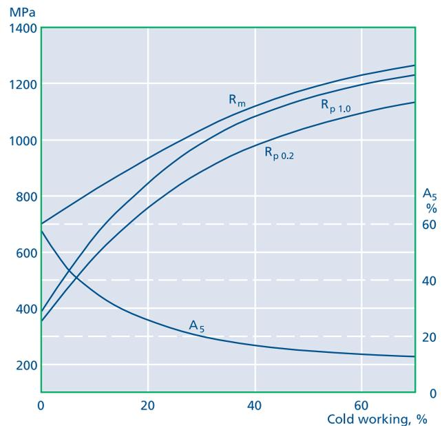
Fig. 12. 254 SMO® – influence of work hardening on strength properties.
