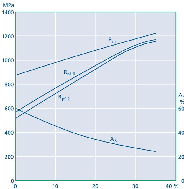
Fig. 13. 654 SMO® – influence of work hardening on strength properties.
