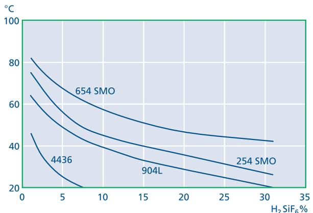
Fig. 5. Isocorrosion curves, 0.1 mm/y, in pure fluosilicic acid.
